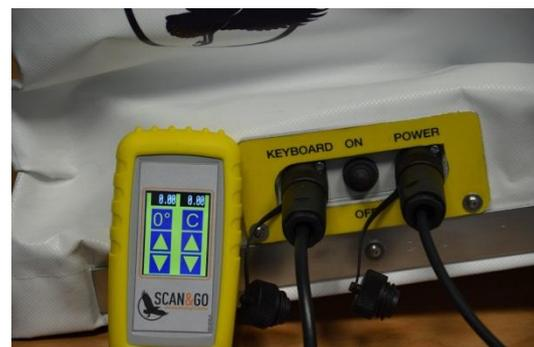
Pressing the button with the indication 0°, the system proceeds automatically reaching the horizontal plane on both axes.
