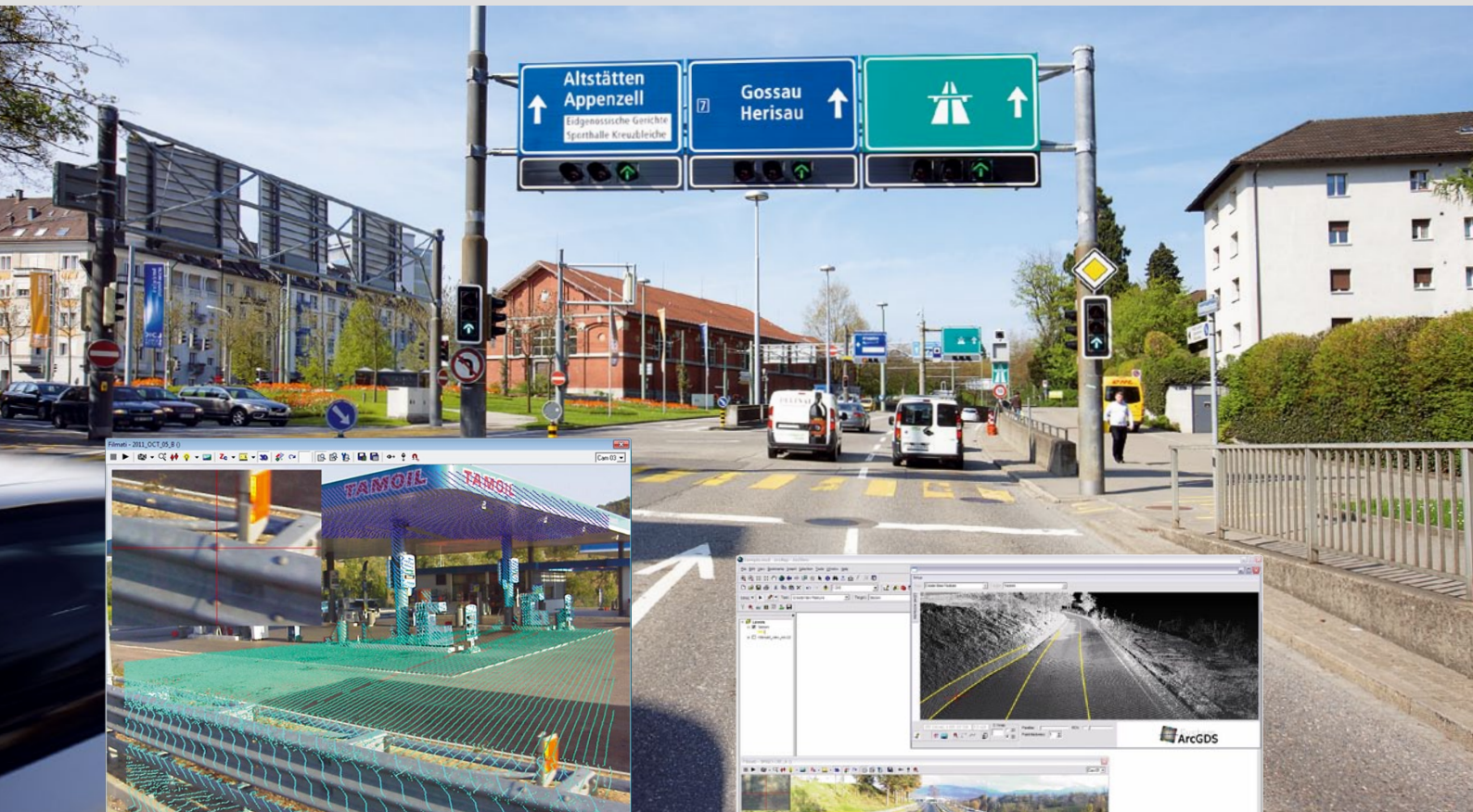
Leica Pegasus:One marries image and lidar data together into a GIS-enabled interface.
