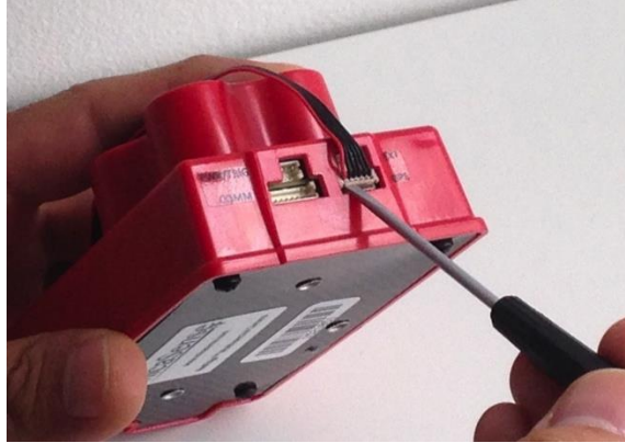
Figure 17: Removal of Connectors Using Small Flathead Screwdriver
